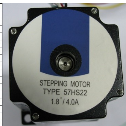
E.g.1: Driver nameplate 1 E.g.2: Driver nameplate 2 Motor nameplate / stepper angle = 1.8^\circ
