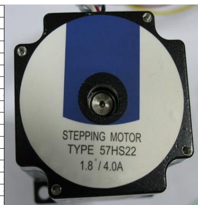
Motor nameplate/ stepper angle=1.8°
