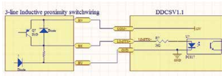
Picture 2-15 Inductive proximity switch wiring mode
