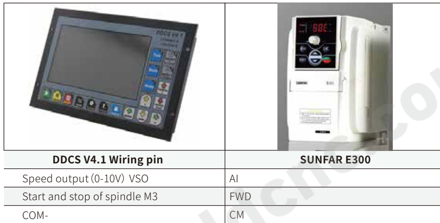
Figure 2-9 DDCS and VFD wiring
