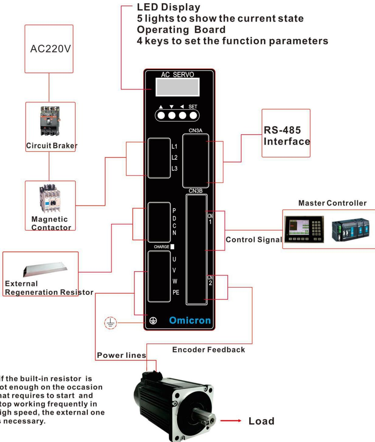
if the built-in resistor is not enough on the occasion that requires to start and stop working frequently in high speed, the external one is necessary.
