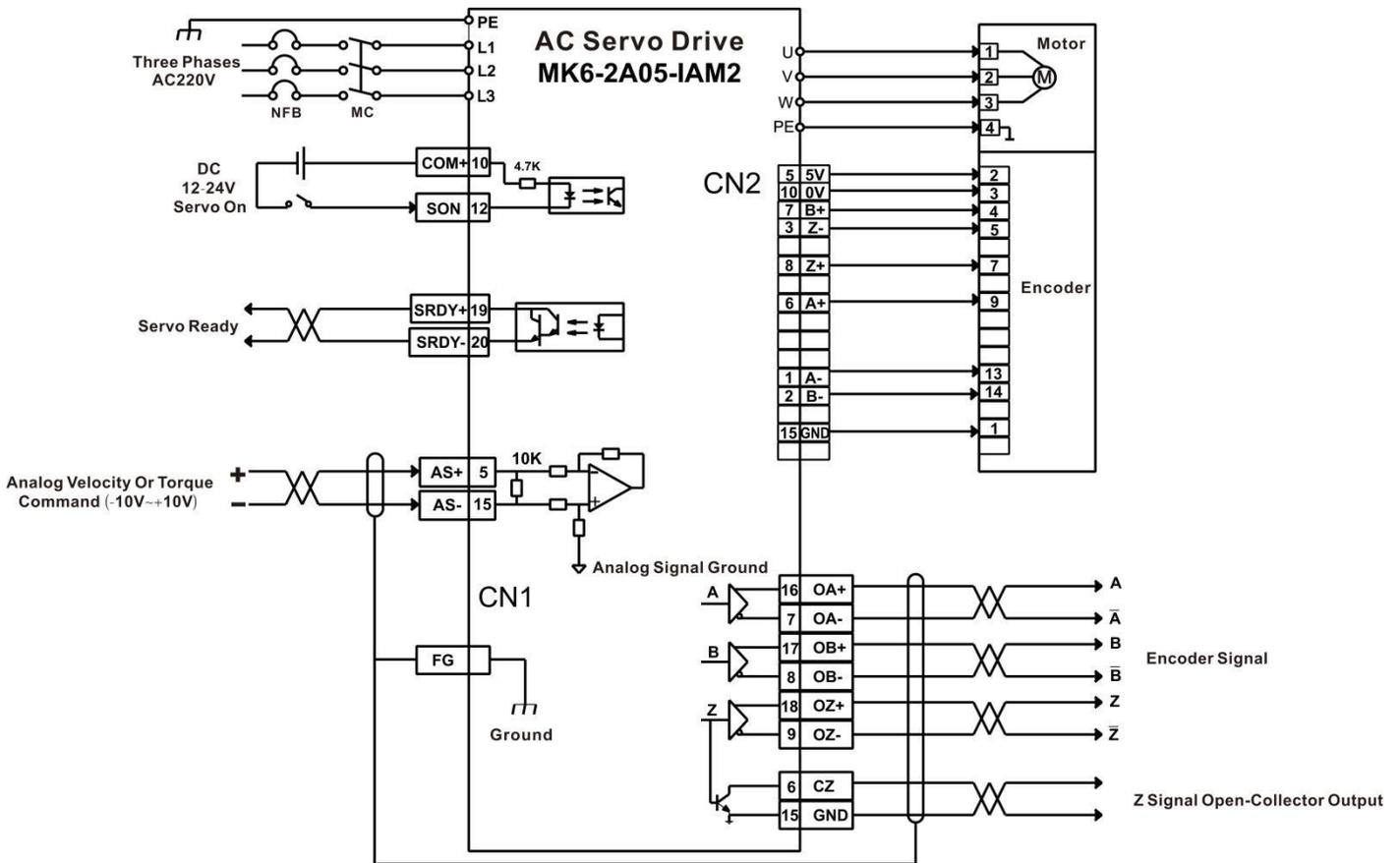
The wiring example (above) is for servo motors with flange size 60mm, 80mm and 90mm. When connected with servo motors with flange size 110mm and 130mm, please connect as following:
