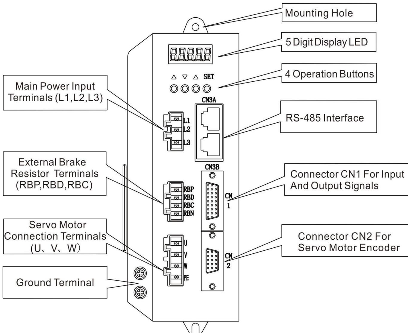
“SET” Button: Enter the parameter settings or set the values to select parameters and exit.
