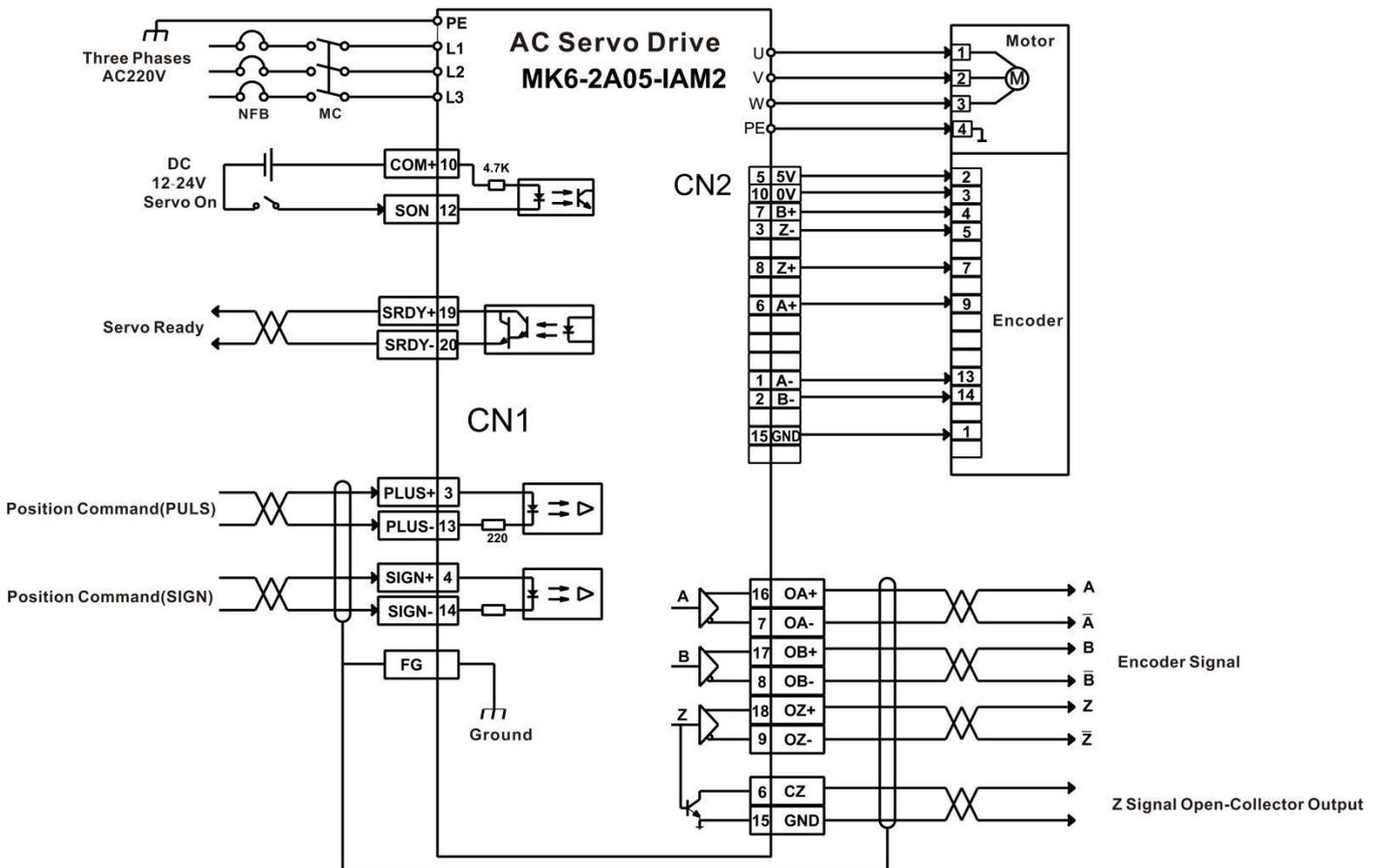
The wiring example (above) is for servo motors with flange size 60mm, 80mm and 90mm. When connected with servo motors with flange size 110mm and 130mm, please connect as following:
