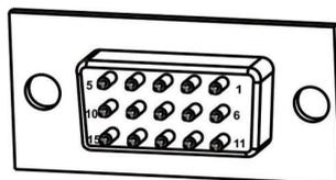
Connector CN2 Soldering view
