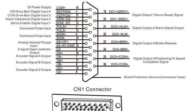
Connector CN1 Soldering view
