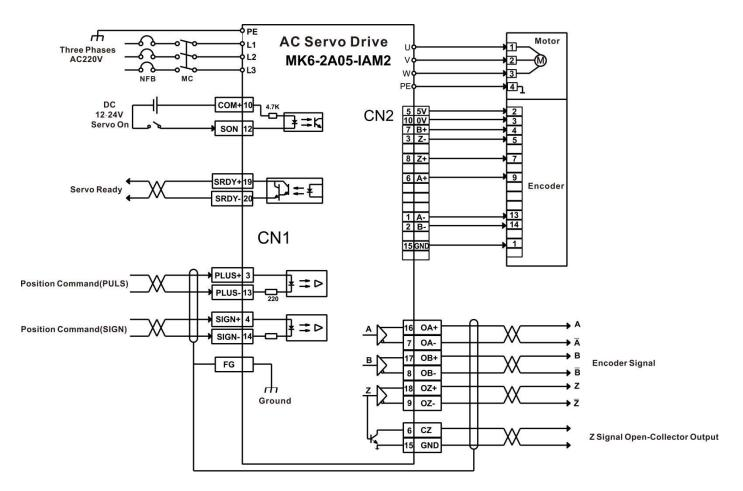
The wiring example (above) is for servo motors with flange size 60mm, 80mm and 90mm. When connected with servo motors with flange size110mm and 130mm, please connect as following:
