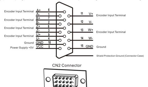
Connector CN2 Soldering view
