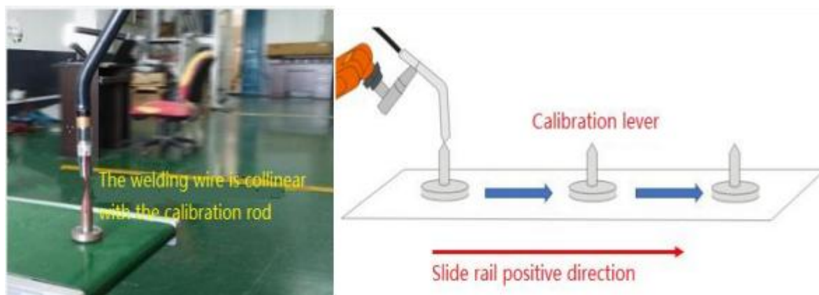
Figure 13.2 New Calibration Point
