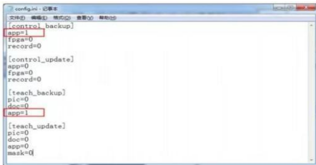
Figure 9.3 Configuration file setting parameter backup system program
