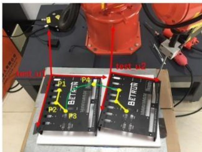
Figure 16.2 Example of "User Coordinate System Transformation" command
