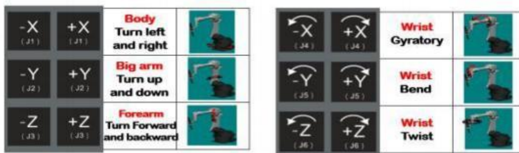
Figure 3.3 Keys function when the operation type is "joint coordinate system"
