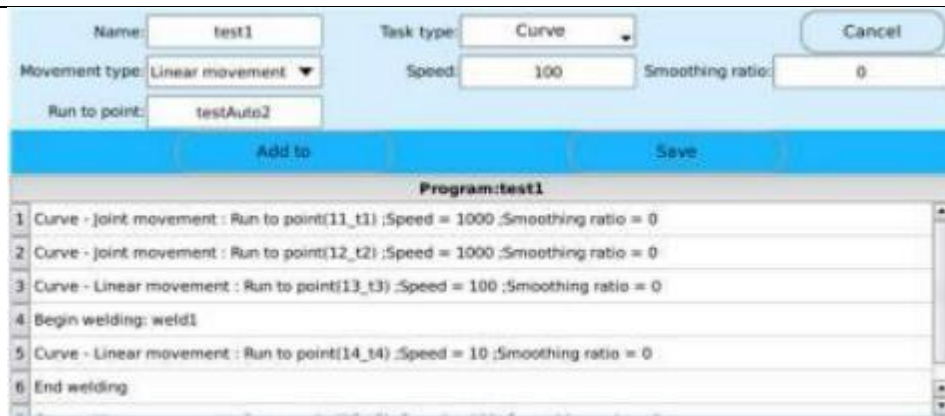
Figure 5.2 Basic program editing interface
