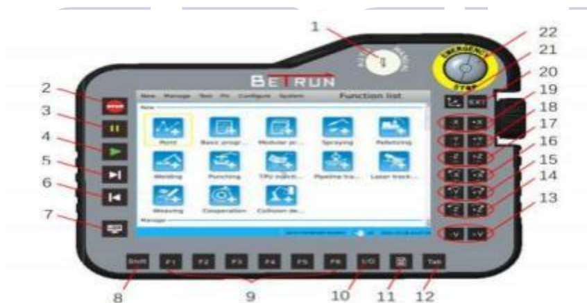
Figure 1.3 Front appearance of the teach pendant
