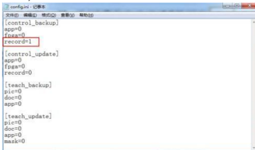
Figure 9.5 Configuration file backup controller user program
