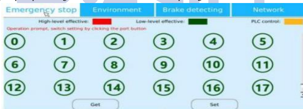
Figure 8.4 Emergency stop output configuration
