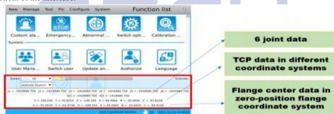
Figure 4.3 Real time display of current "point" information
