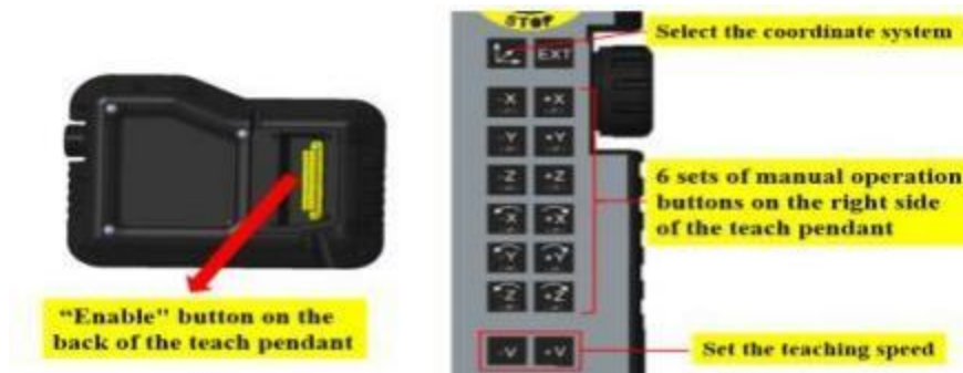
Figure 3.1 Buttons for manual teaching
