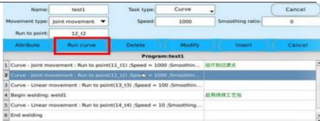
Figure 5.7 [Run curve] button will appear when selecting curve command
