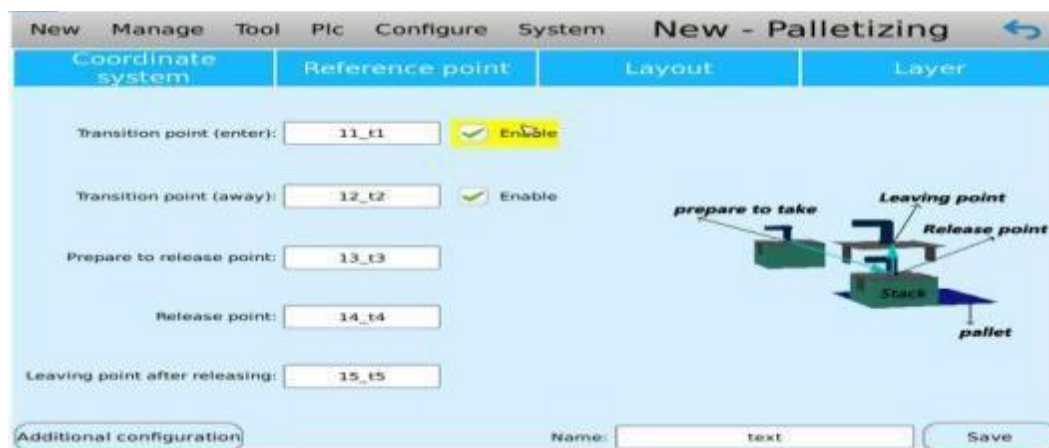
Figure 17.6 Reference point setting
