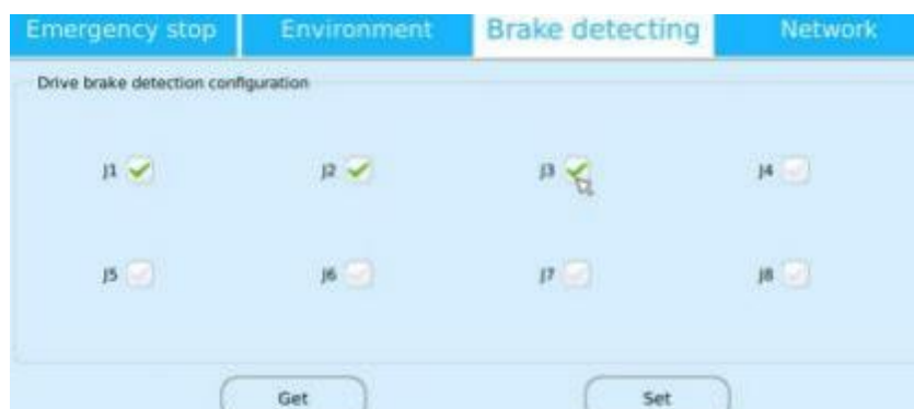
Figure 8.7 Brake abnormality detection attribute setting
