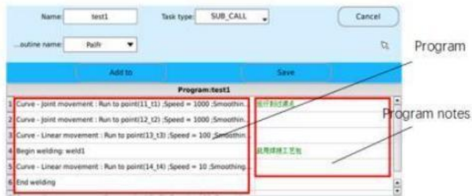
Figure 5.3 Program content and annotation display
