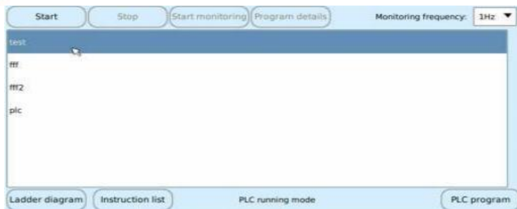
Figure 6.3 PLC program execution interface
