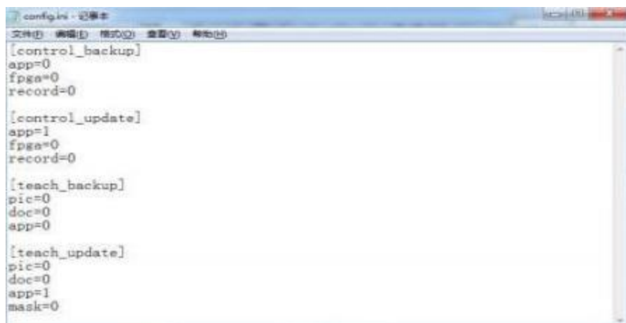
Figure 9.10 Configuration file setting parameter update exe program
