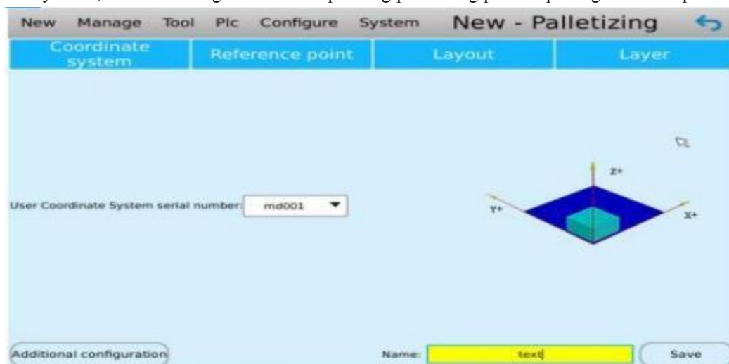
Figure 17.5 Select user coordinate system
