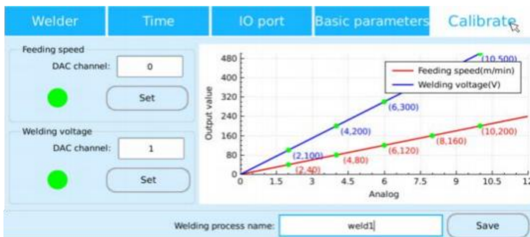
Figure 18.7 Current and voltage calibration
