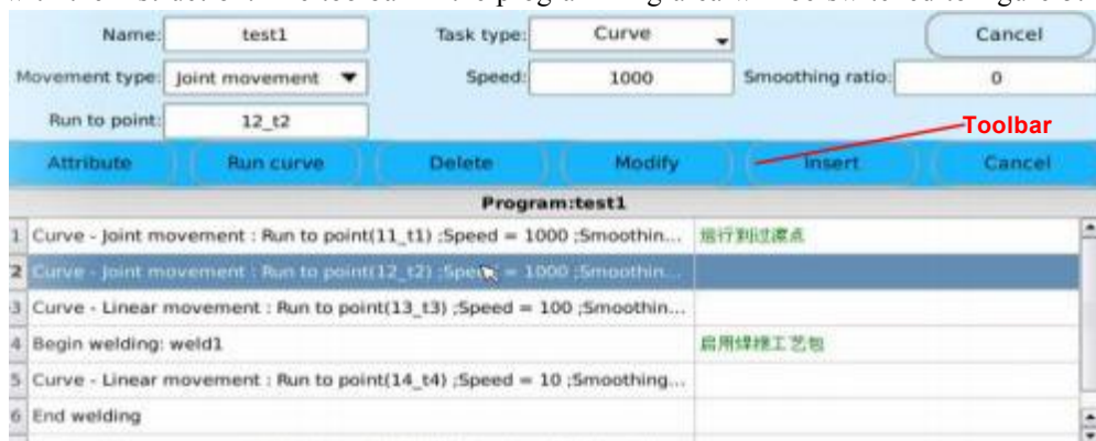
Figure 5.4 Toolbar in the programming area
