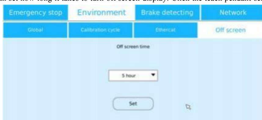
Figure 8.6 Off screen time configuration
