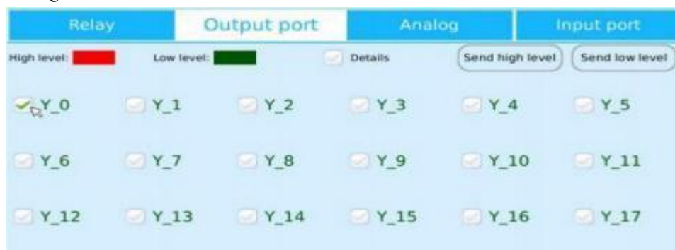
Figure 7.6 Set output port
