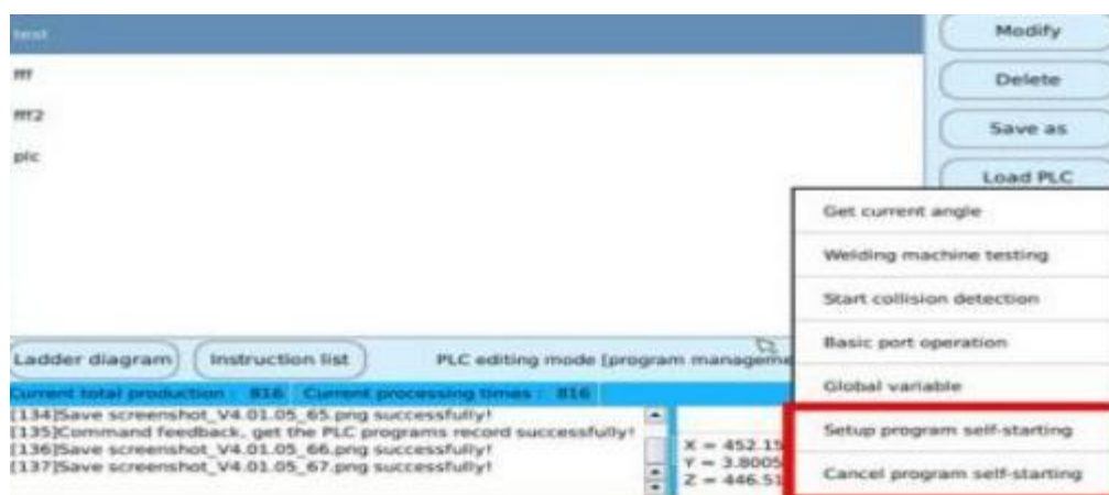
Figure 6.4 Setting the automatic operation of PLC program
