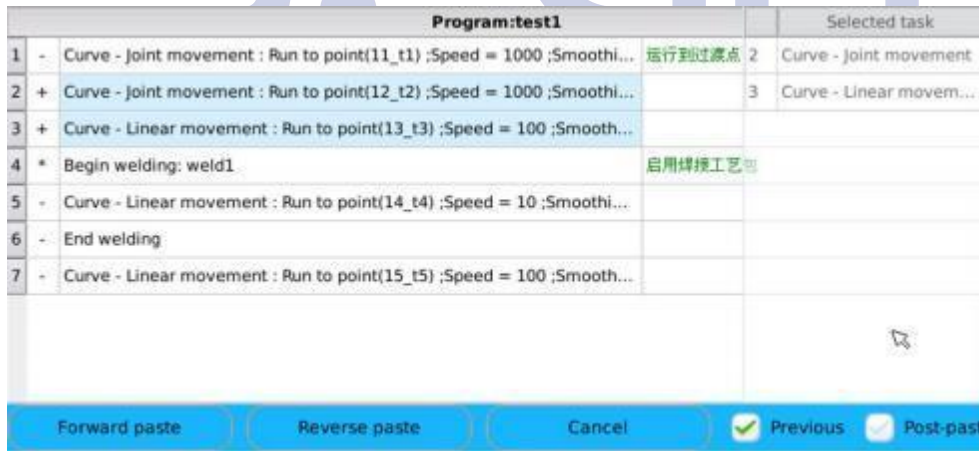
Figure 5.6 Forward or reverse pasting instructions at the specified position
